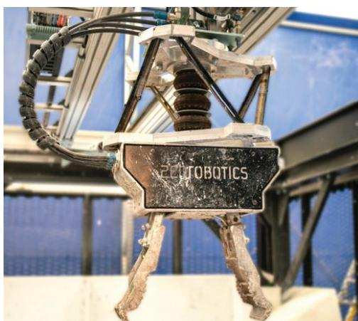
Figure 54 : Pince du robot Heavy Picker (source: ZenRobotics)
