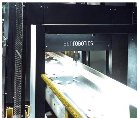
Figure 53 : robot Fast Picker (source: ZenRobotics)
